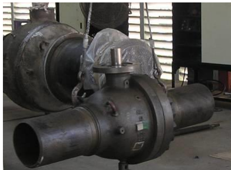
Fig.3. Handling a valve with welded pup piece.
