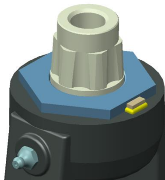
Figure 42 - Tab Welding of Yoke Sleeve Nut
