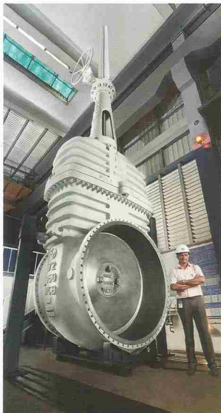
72 inch Class 150 gate valve. One of the largest cast steel gate valves manufactured in India.
