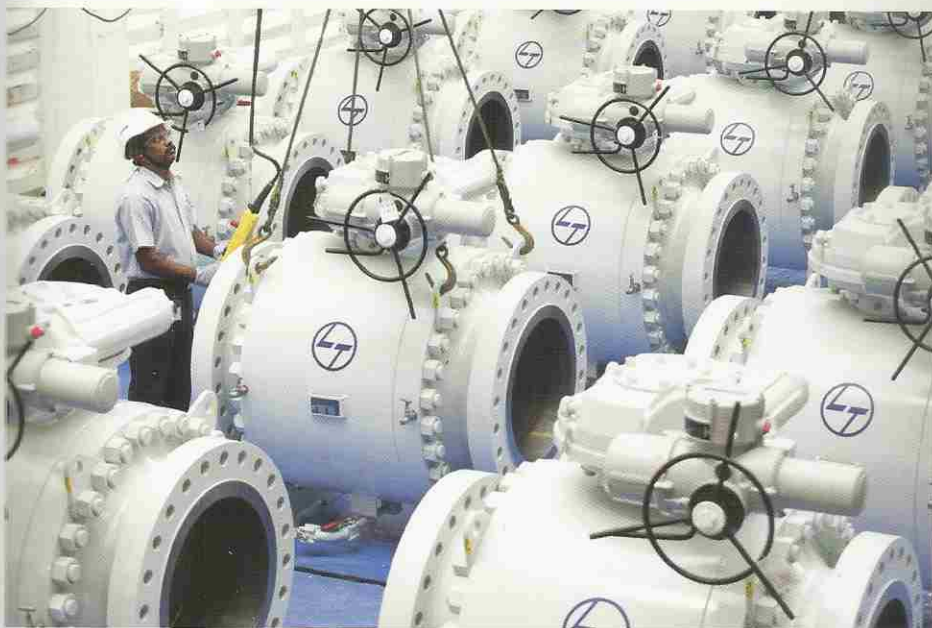
L&T Valves’ trunnion-mounted ball valves conform to API 6D standard. Available in ASME classes from 150 to 2500, in 2-piece and 3-piece designs, in both bolted and welded constructions and in sizes up to 56 inches, these valves have a proven track-record in pipeline applications.
